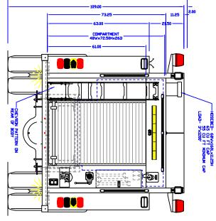
6. THE EFFECTIVE DOOR OPENINGS WILL BE APPROX. 2" LESS THAN THE NOTED COMPARTMENT OPENING FOR ROLL UP DOORS AND UP TO APPROX. 4" LESS FOR HINGED DOORS
